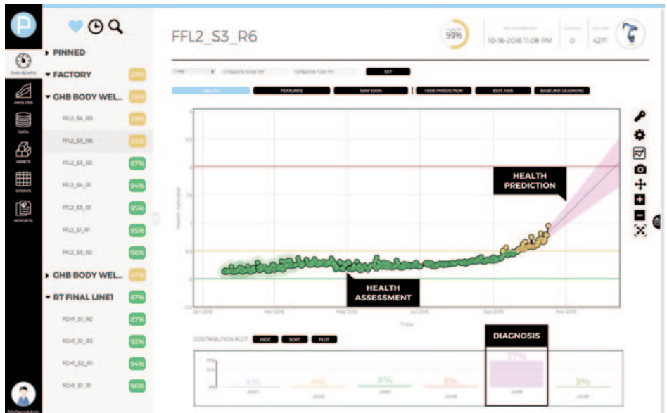
Fig. 4—A comprehensive smart-factory digital strategy revolves around plant-floor connectivity and data ingestion to machine-monitoring and predictive-maintenance technologies. Such a setup can provide early fault detection and prediction, and assist manufacturers in using AI tools to transform maintenance activities from a “fail and fix” to a “predict and prescribe” paradigm.
